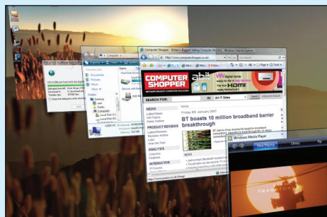
▲ Flip 3D throws your windows into 3D space to make it easy to find the one you're looking for
